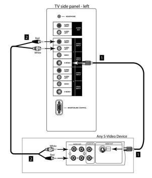
Figure 10. Connecting an S-Video Device.
